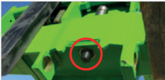
Tac-Lock: hydraulic attachment clamping system from the cab
