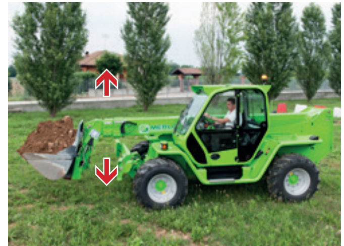
BSS hydro-pneumatic boom suspension (opt) engaged by the operator, it speeds up transfer, protects the load and improves productivity.. It is deactivated at speeds <3 km/h.
