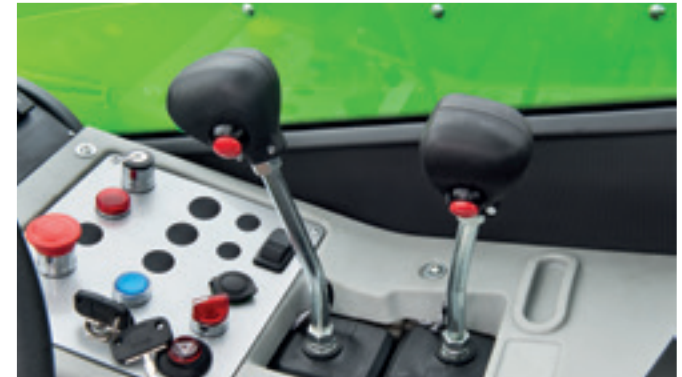
Basic Version: levers for operating the boom, carriage, attachments and boom side shifts
