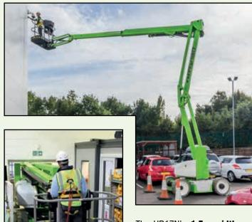
The HR17N's 1.5m width and sub 2m height enables travel restricted spaces. through Optional non-marking tyres mean that it can work both inside and out making it ideal for industrial or maintenance work.
