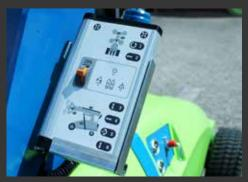
Multifunction control panel in operatorfriendly design with integrated buttons and signal lights, Double action safety keys and Gyro funtionality are both in the standard setup on the winlet 575.
